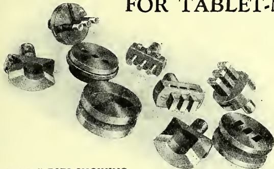
PUNCHES & DIES SHOWING VARIOUS SHAPES AND SIZES
